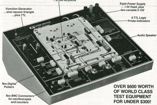
Here's PB-503, the total design workstation. It has everything! Instrumentation, including a function generator with continuously variable sine/square/triangle wave forms—plus TTL pulses. Breadboards with 8 logic probe circuits.
