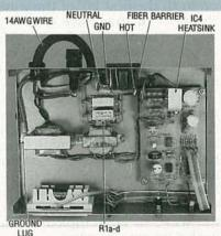
FIG. 5—HERE IS THE FINISHED prototype. It's a good idea to use standoffs to mount the transformers so that R1-a—d's connections are adequately spaced from the case. The author also used a fiber barrier between the PC board and the AC socket for added protection.
