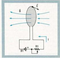
FIG. 2—SELF INDUCTANCE OF A COIL. As the current I changes the magnitude of B, the magnetic flux  $\Phi$  enclosed by the coil also changes proportionately. An electromotive force and associated E field results that tends to oppose the change in I and keep the flux constant. The inductance is the ratio of the change in flux to an infinitesimal change in current. It is related to the geometry of the coil and any material present within that coil.
