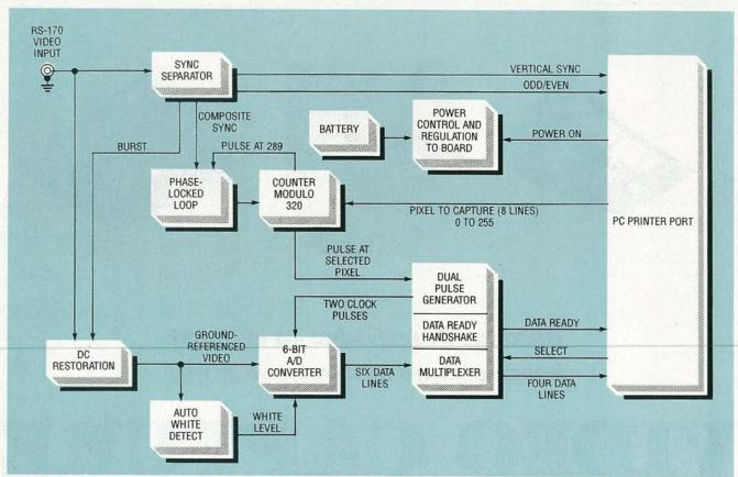
FIG. 1—BLOCK DIAGRAM of the image capture board.
