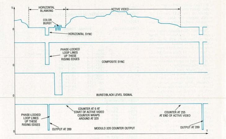
FIG. 3—WAVEFORMS SHOW THE significance of count 289 being returned to the PLL for horizontal-sync alignment.
