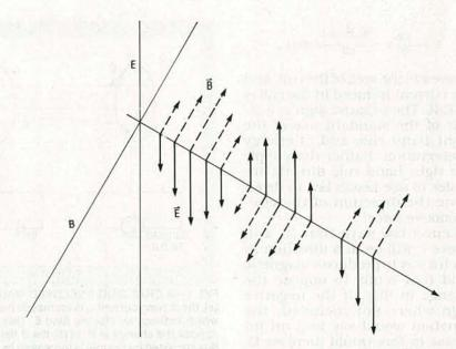
FIG. 3—AN ELECTROMAGNETIC WAVE in empty space. A few of the E-field vectors, shown as solid arrows, and B-field vectors, shown as dashed arrows, that simultaneously change magnitude at each point as the wave propagates through space.
