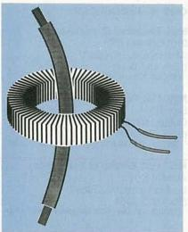
FIG. 4-A TOROIDAL CURRENT transformer is economical and accurate. It is also self-shielding. But you physically have to disconnect and thread the primary wire through the core center.
