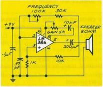
FIG. 1—TO TRACK CABLES electronically, you can use this circuit. The LM386 is set up as a simple oscillator and the potentiometers adjust the frequency and gain.
