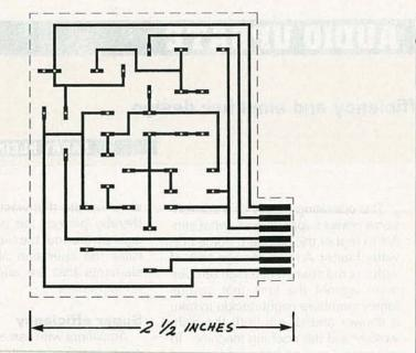
FIG. 4—THE FOIL PATTERN for our regulator circuit. It's shown here actual size.
