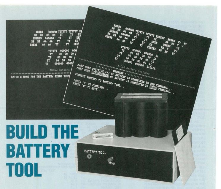
Get the most out of your rechargeable batteries with this microcontrollerbased battery discharger.
