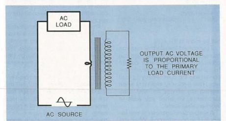
FIG. 3—A CURRENT TRANSFORMER is just a transformer that has a very low-impedance primary (often ONE turn or less) and a high step-up ratio. The voltage across the secondary is proportional to the primary current.
